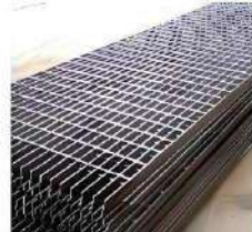
Plat Grating Material Besi, dgn Hot deep Galvanis Tebal 4.5 & 5mm Tinggi 25 & 32 mm Uk. 900 x 6.000 mm Clamp type A,B, C
